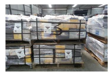
Note the Horizontal strap to each layer of ULAB, two vertical straps secure the ULAB to the pallet, clear plastic stretch wrap, and pallets in good condition
